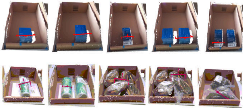
Figure 22: Examples of grasp pose estimations on DARKO objects, visualized as coloured point clouds. The top row shows objects in different configurations, while the bottom row presents the same objects wrapped in transparent plastic bags. Red markers indicate the selected grasp poses. In all cases, the grasp predictions are generated directly from point cloud data.
