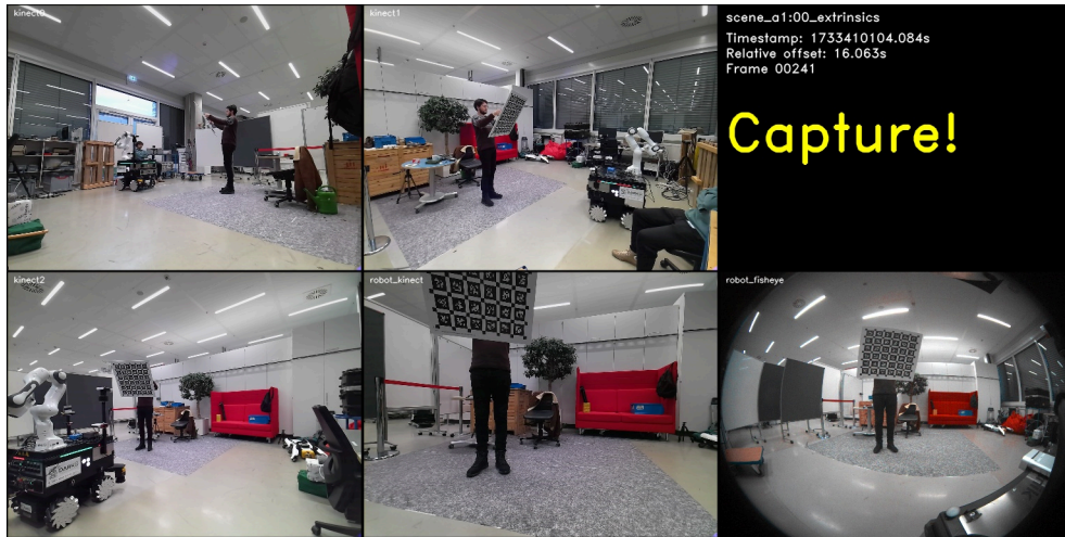
Figure 6: The user interface shows an operator recording calibration images in a synchronized multi-camera setup involving the DARKO robot platform (lower left). The operator prompts image acquisition during steady poses via speech commands, while having their hands free to securely hold and move the calibration target. The recognized spoken trigger word is shown on the right in yellow.
