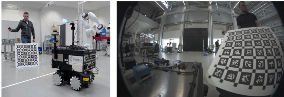
Figure 4: For intrinsic and extrinsic camera-to-camera calibration, we use an AprilGrid calibration target in combination with a commercial calibration software toolkit.
